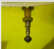
Getto rotante lava cisterna Internal nozzle for tank washing Injector interno lava tanque
