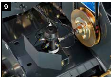
9 BEKA-MAX continuous chain oiling system
