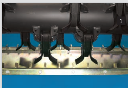
Contro-coltelli speciali a denti seghettati Special notched toothed counter-knives Contra-cuchillas especiales dentadas
