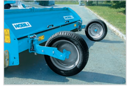
Ruote sterzanti: 185/60-14 BK 230/280 e 195/65-15 BK 320 Steering wheels: 185/60-14 BK 230/280 and 195/65-15 BK 320 Ruedas móviles: 185/60-14 BK 230-280 y 195/65-15 BK 320
